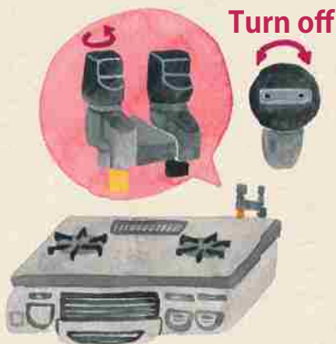
Main gas supply tap
