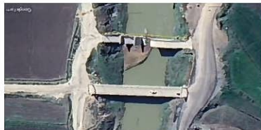
Bridge collapse due to pier settlement due to ground failure (Antakya)
