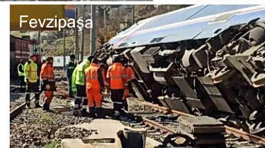
Buckling of rails due to faulting and ground deformation, toppling of trains
