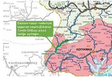
Location of Erkenek tunnel Old Erkenek Tunnel is 330m long and unsupported New Erkenek Tunnels are 1816 m long
