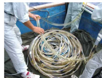
Boomer + 12channel short streamer cable
