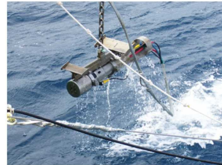
Air Gun + Single channel streamer cable
