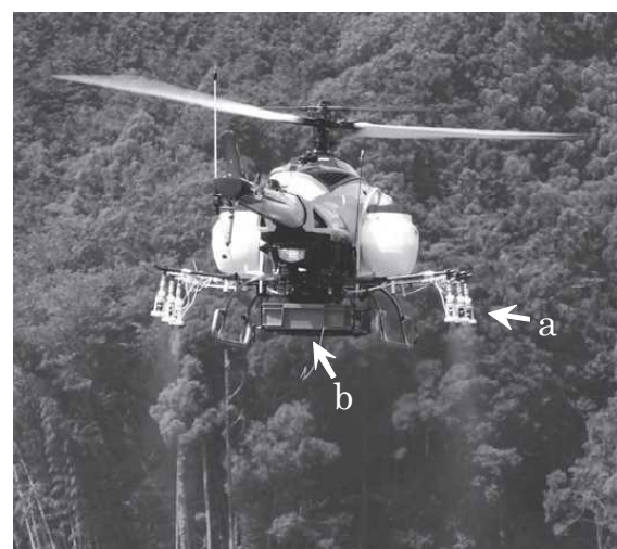
Fig.1 Prototype of electrostatic spraying system for unmanned industrial helicopter. a: Electrostatic spray nozzle, b: High voltage power supply
